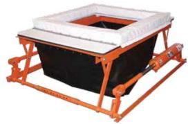
Installed between the tracks, Boot-Lift® Connectors form the link between the railcar and a plant's under-track conveying system. Powered by an air-over-hydraulic system, the unloading boots rise to the gates for clean, efficient and safe unloading of bottom discharge hopper cars. By funneling material to the under-track system, Boot-Lift® Railcar Connectors prevent material from being blown away by wind while eliminating the safety hazard of requiring workers to crawl under the car.
